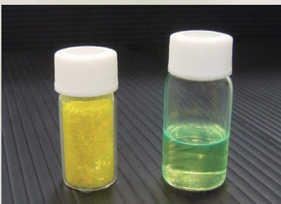
The "PXX derivative" high-performance organic semiconductor material developed by Sony. On the left is the powder form used in the development effort described here. On the right is an ink-solution with a "PXX derivative" for use in future printing processes.
