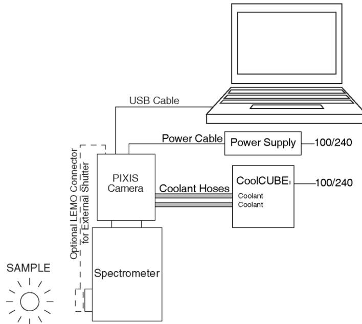
Figure 5. Typical Spectroscopy Experiment Layout (Liquid-cooled Camera with CoolCUBE<sub>II</sub>)
