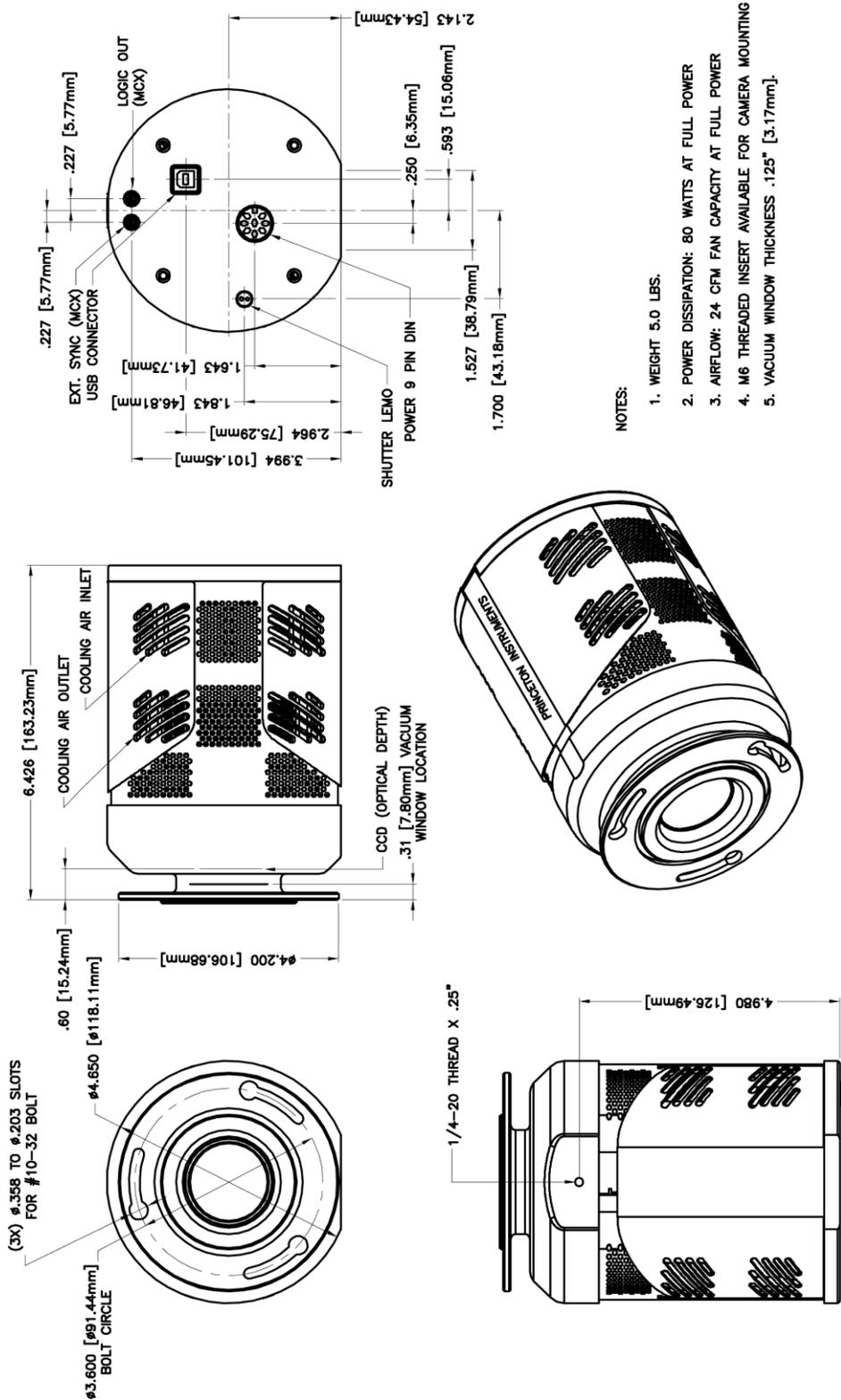
Figure 66. Spectroscopy-Mount: No Internal Shutter, 3.60 bolt circle (Air-cooled)
