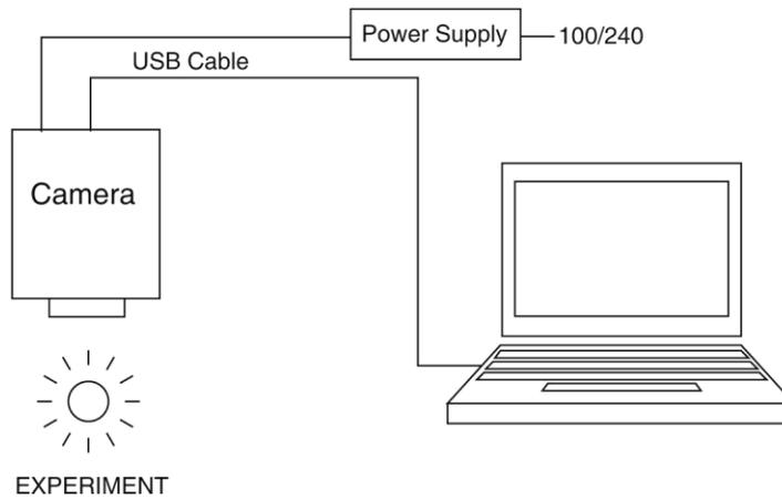
Figure 2. Typical Imaging Experiment Layout (Air-cooled Camera)
