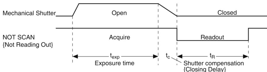
Figure 22. Exposure of the CCD with Shutter Compensation
