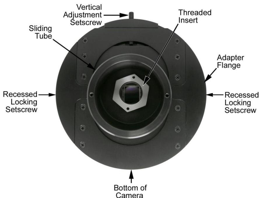
Figure 10. Adjustable C- to Spectroscopy-Mount Kinetics Adapter
