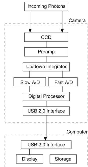
Figure 12. Block Diagram of PIXIS System
