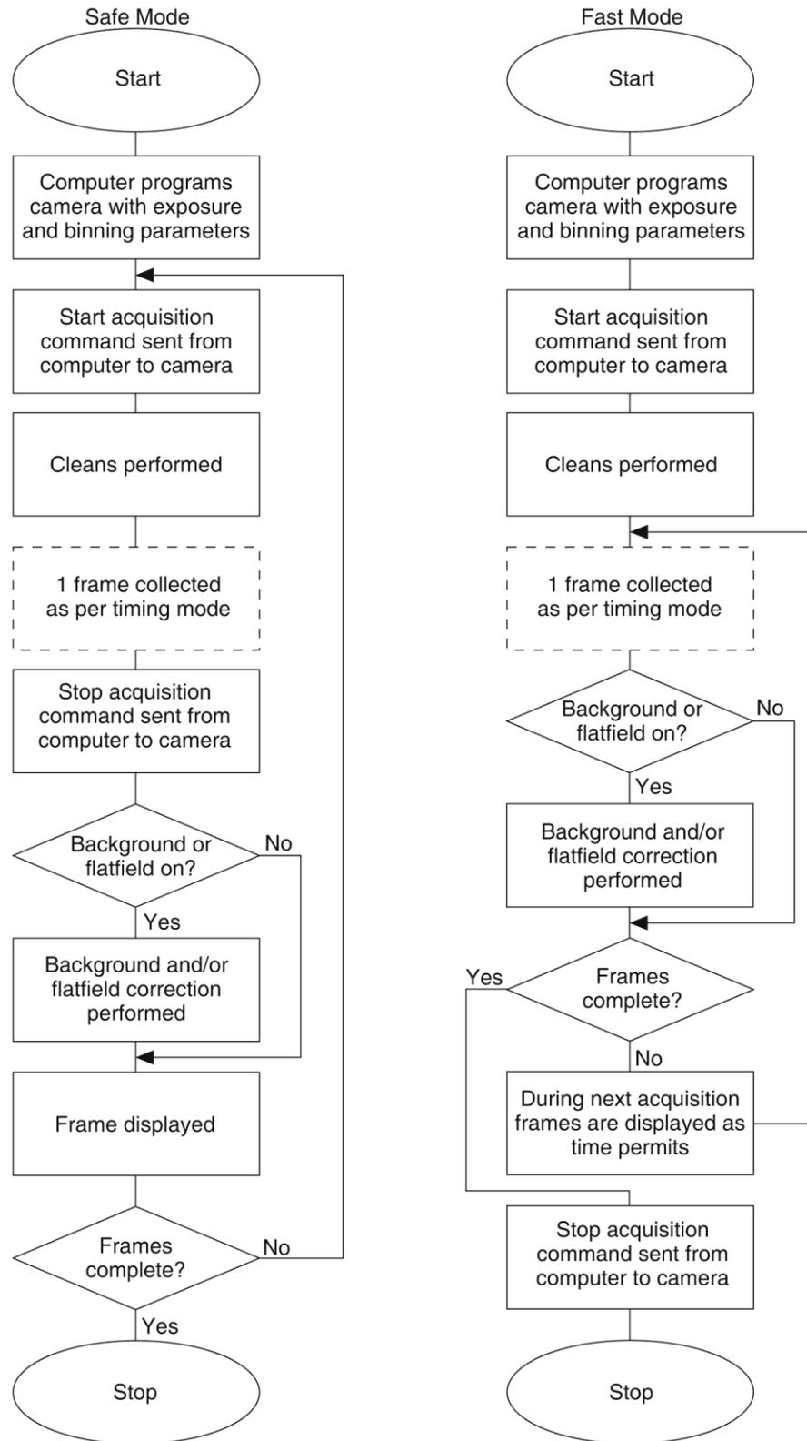
Figure 36. Chart of Safe and Fast Mode Operation
