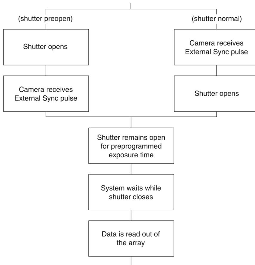
Figure 30. Chart Showing Two External Sync Timing Options
