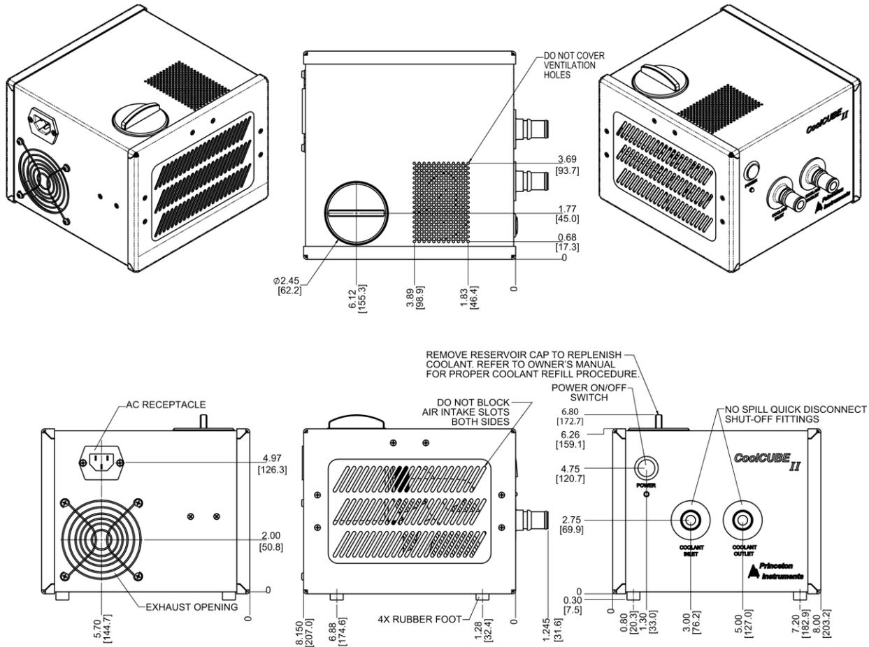
Figure 69. CoolCUBE<sub>II</sub> Circulator
