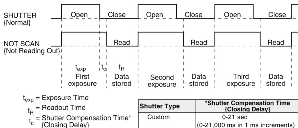
Figure 29. Free Run {No Response} Timing Diagram
