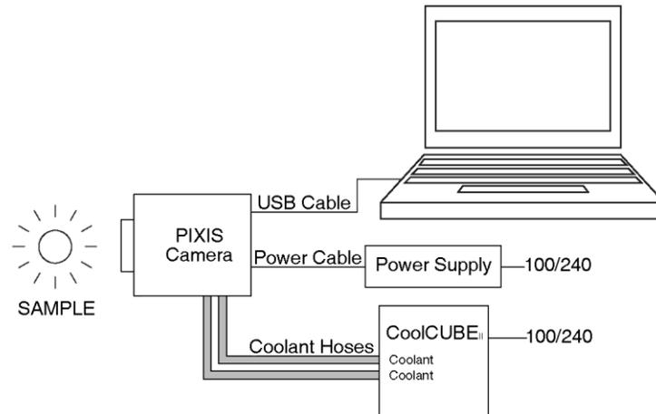
Figure 4. Typical Imaging Experiment Layout (Liquid-cooled Camera with CoolCUBE<sub>II</sub>)
