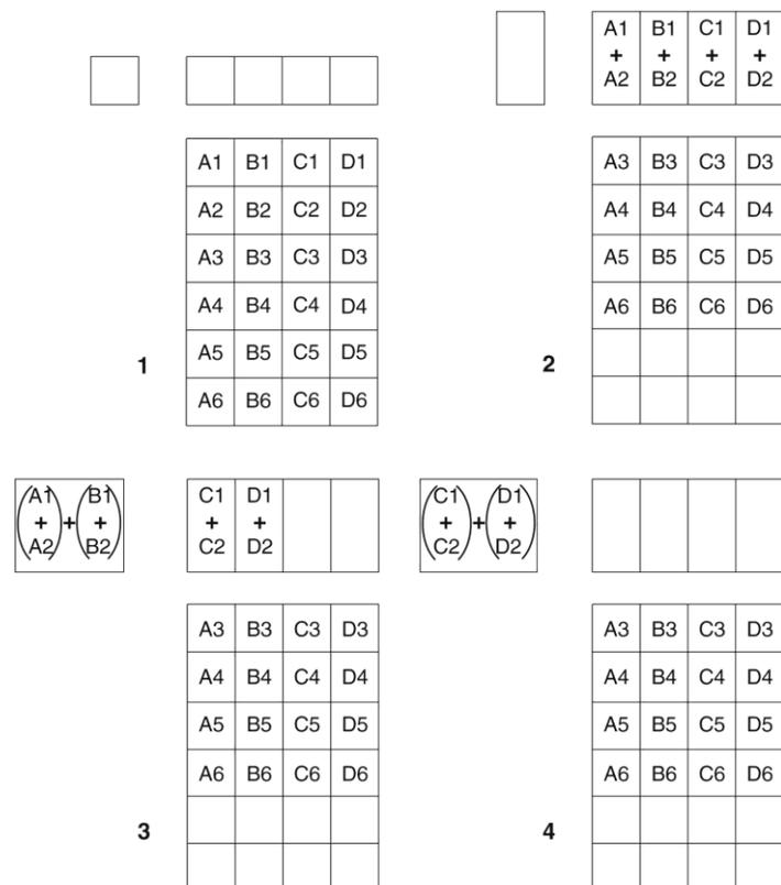
Figure 26.  $2 \times 2$  Binning
