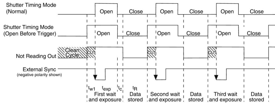
Figure 34. LightField Clean Until Trigger (CUT) Timing Diagram
