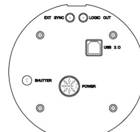
**Shutter:** LEMO<sup>®</sup> connector provides the shutter drive pulses for driving a Princeton Instruments-supplied external shutter (for example, a shutter at the entrance slit of a spectrograph). Camera power must be OFF before connecting to or disconnecting from this connector.
