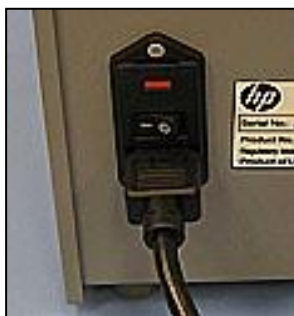
Figure 6-4 On/off switch on rear of dispenser. Depress “1” to turn on.
