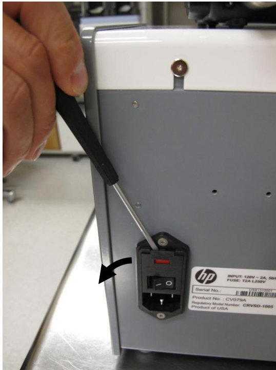
Figure 6-5 Pry the cover at the top of the power inlet module and flip down
