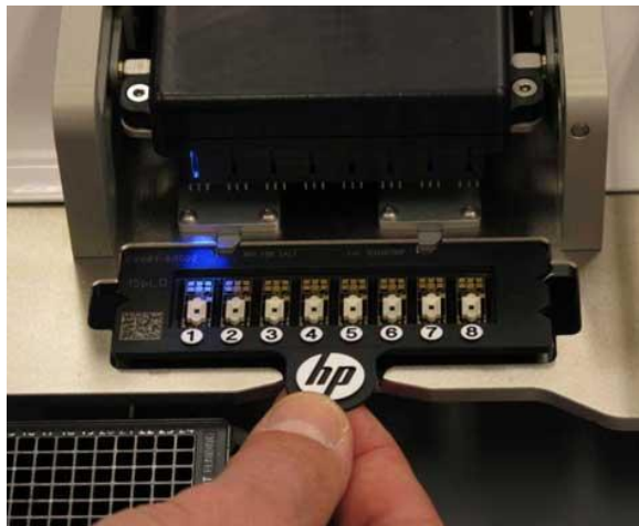
Figure 4-21 Loading a new Dispensehead Cassette
