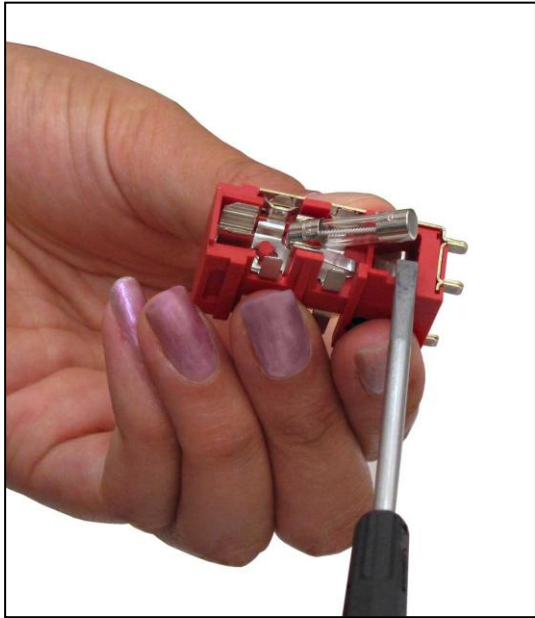
Figure 6-8 Pry the fuse out carefully
