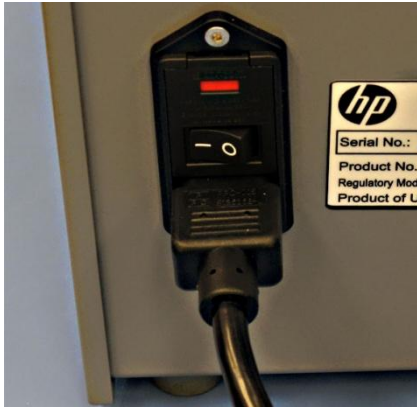
Figure 4-32 On/off switch in the ON position
