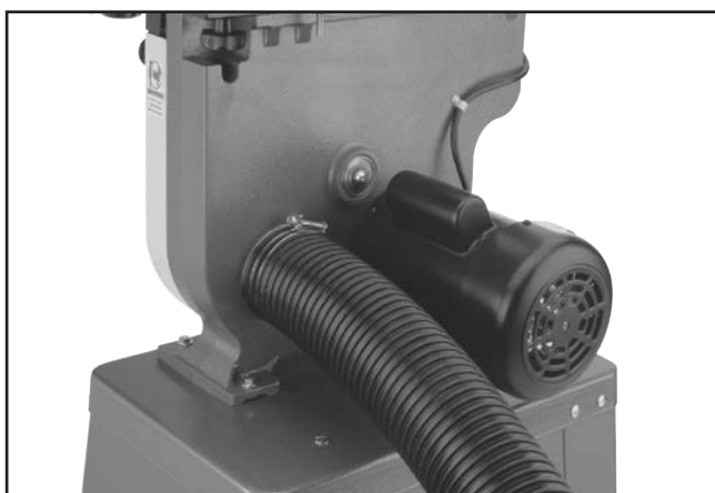
Figure 16. Dust hose attached to dust port.
