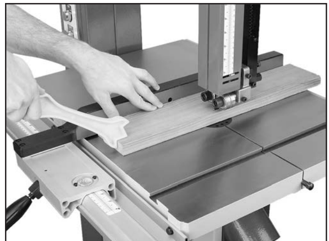
Figure 31. Typical ripping operation.
