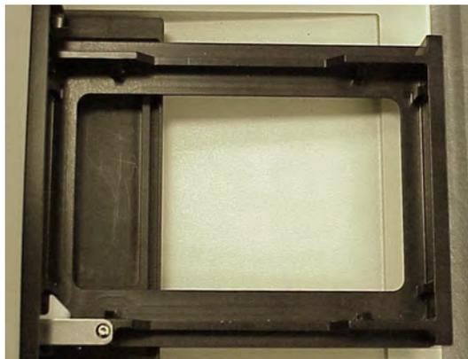
*Figure 4.5: Microplate Drawer without Adapter*
