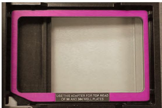
*Figure 2.2: Adapter Inserted in Microplate Drawer*
