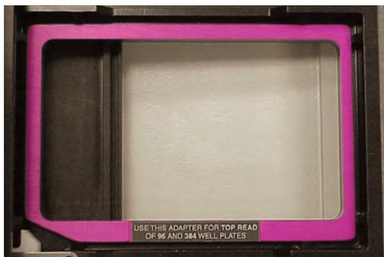
*Figure 4.4: Adapter Inserted in Microplate Drawer*
