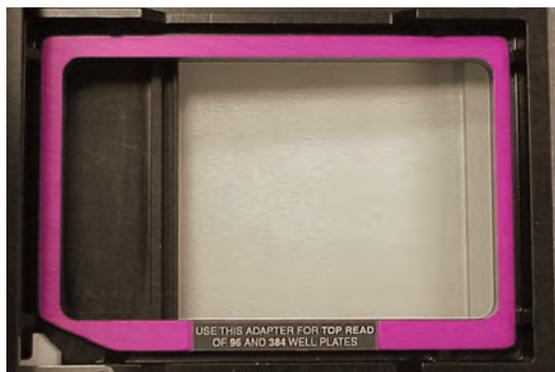
*Figure 1.3: Microplate Drawer (Shown with Adapter Inserted)*
