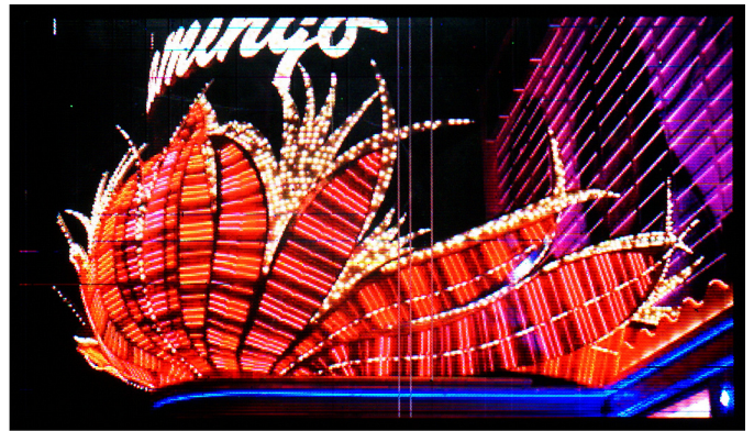
FIGURE 6 — Photograph of 4.1-in. full-color rollable OTFT-driven FWQVGA OLED display.
